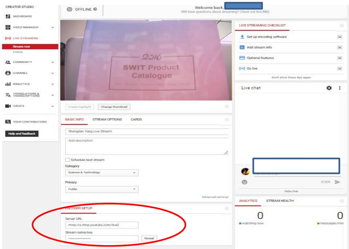
At the bottom of “Stream now” page (red circle), there’s the “ENCODER SETUP” section, in which it contains “Server URL” and “Stream name/key”. Click “Reveal” so you can see the “Stream name/key” for a few seconds.
