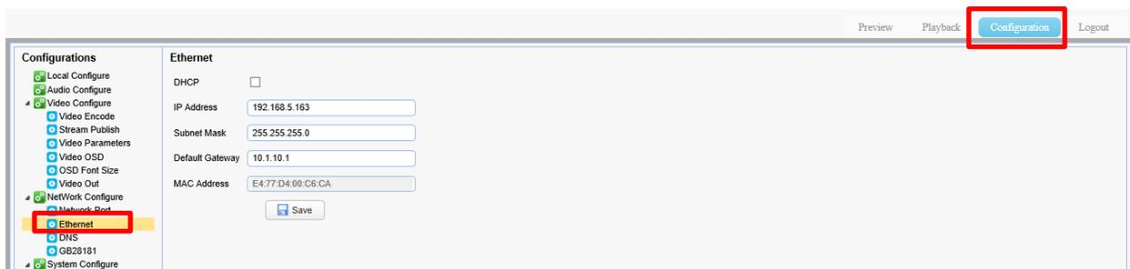
Find the "IP Address" and change it to be consistent with IP1 (router IP). Make sure the first 3 sections are the same. For example, at the beginning of this instruction, notice IP1 is 10.1.10.151, then the user can change the "IP Address" (IP3) to 10.1.10.110. Click on "Save" to save the change.
