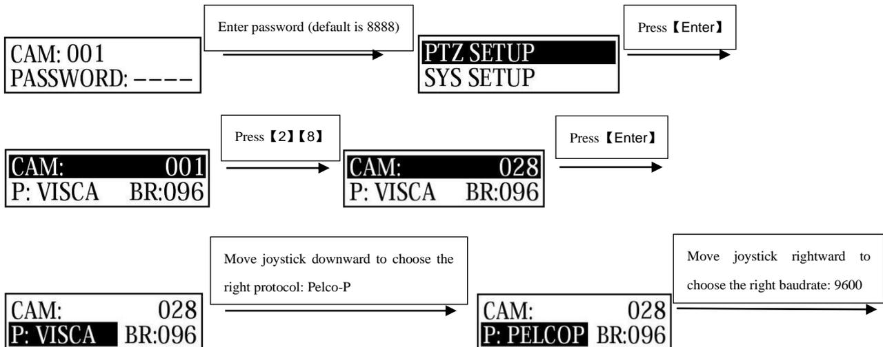
Press **【ENTER】** to confirm the selected baud rate. There will be a 1-sec beep sound once the setup is complete.
